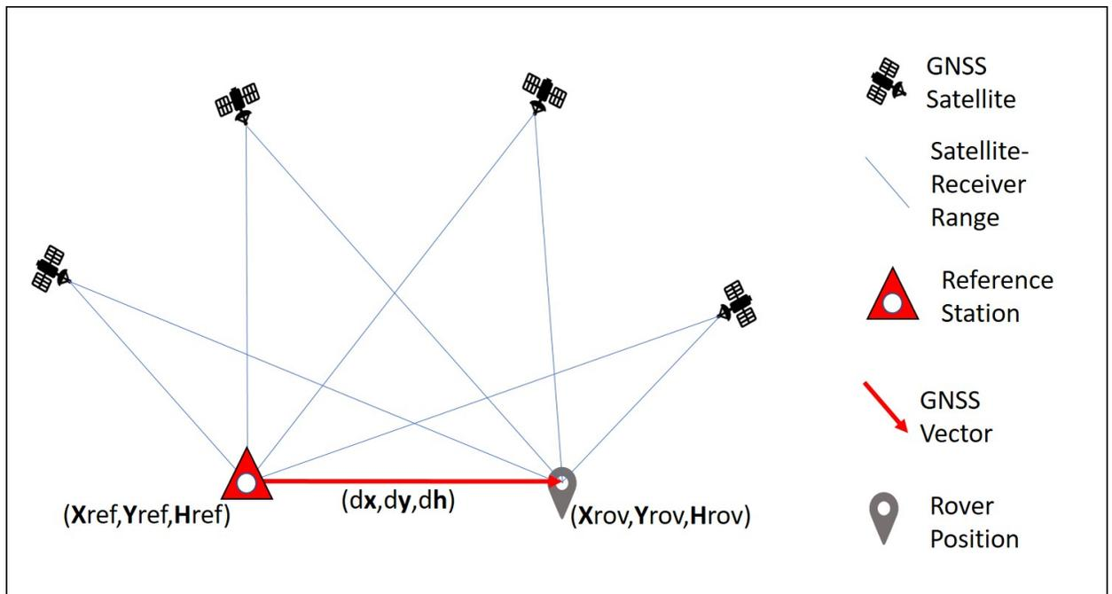
Figure 6: Carrier phase differential GNSS
