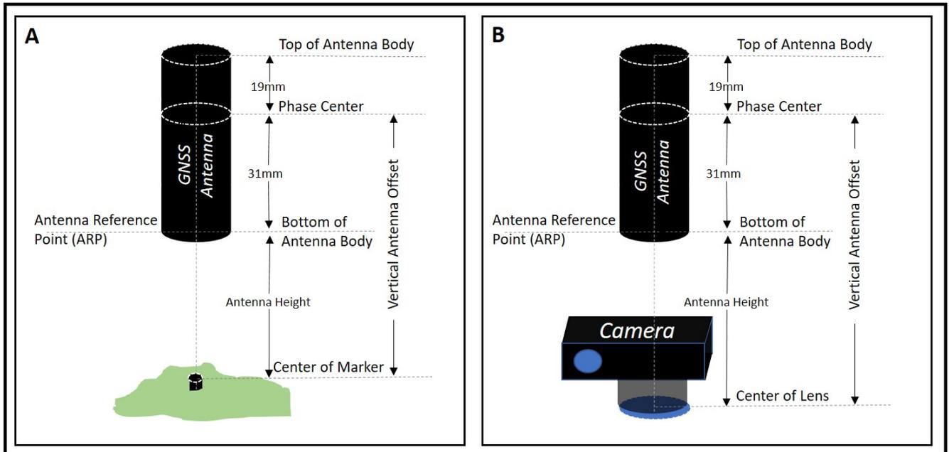
Figure 12: Illustration of Antenna Reference Point (ARP), Phase Center and Antenna Height for occupation of physical marker (A) or when used to survey camera exposure positions (B)
