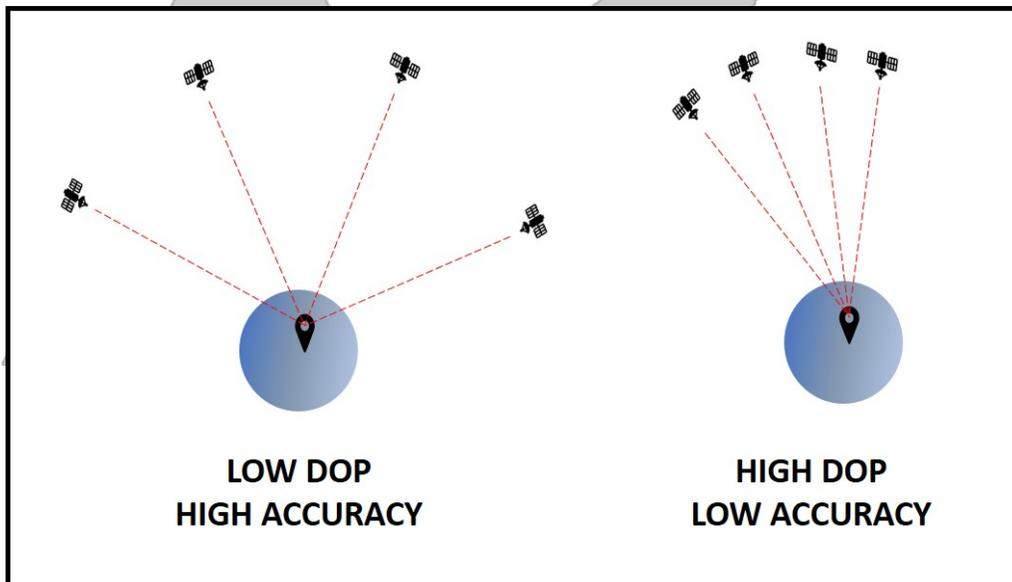
Figure 4: The effects of geometry on accuracy in single point GNSS positioning.
