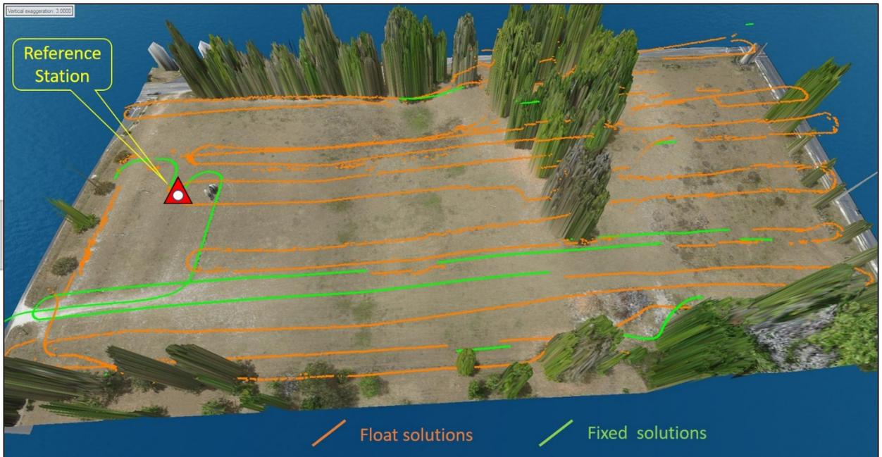
Figure 19: Single frequency PPK GPS results at rover speed of approximately 4m/s. (Approximate field dimensions are 200m x 400 m)
