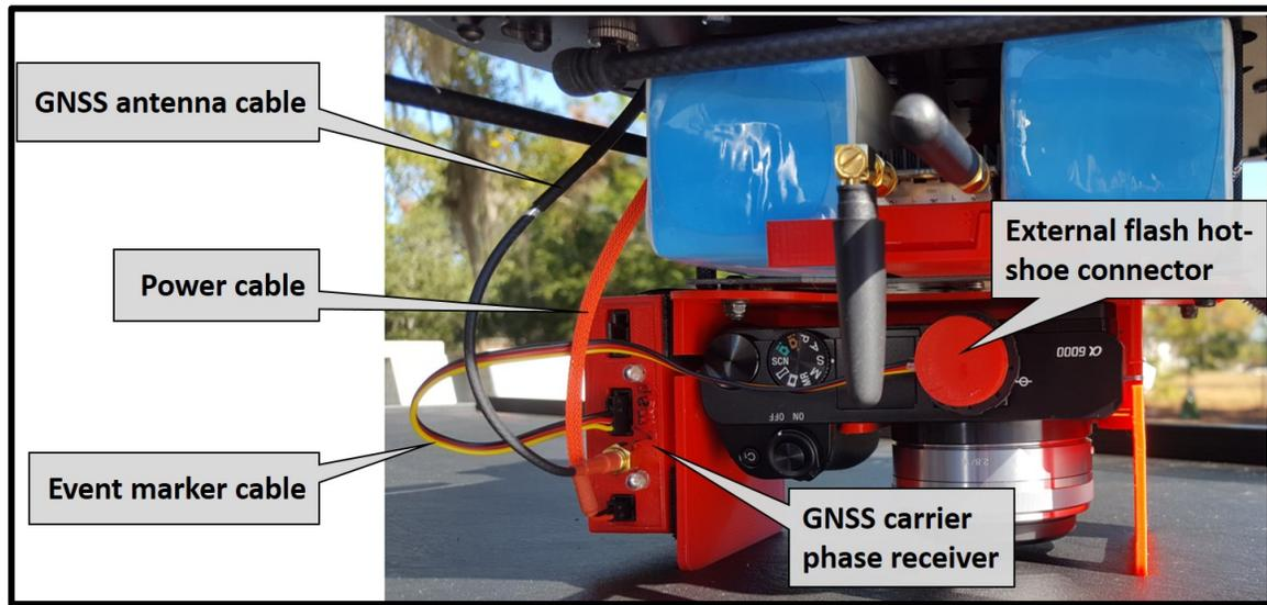
Figure 8: Multirotor platform payload: Camera and dual frequency GNSS receiver capable of event marking.
