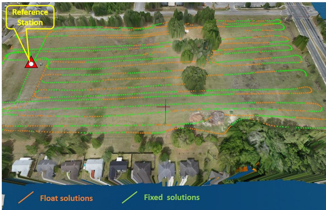
Figure 21: Dual frequency PPK forward GPS results (as in RTK) at rover speed of approximately 4m/s. (Approximate field dimensions are 200m x 400 m)
