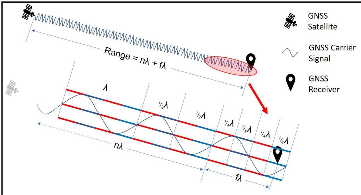
Figure 10: The satellite range expressed in units of wavelengths of the carrier signal.
