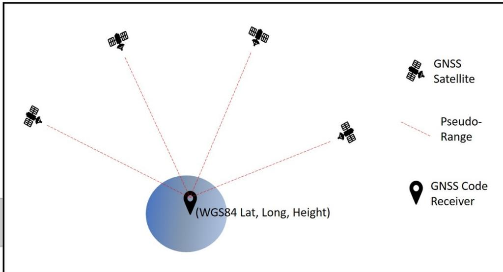
Figure 3: Absolute positioning by means of pseudorangeing
