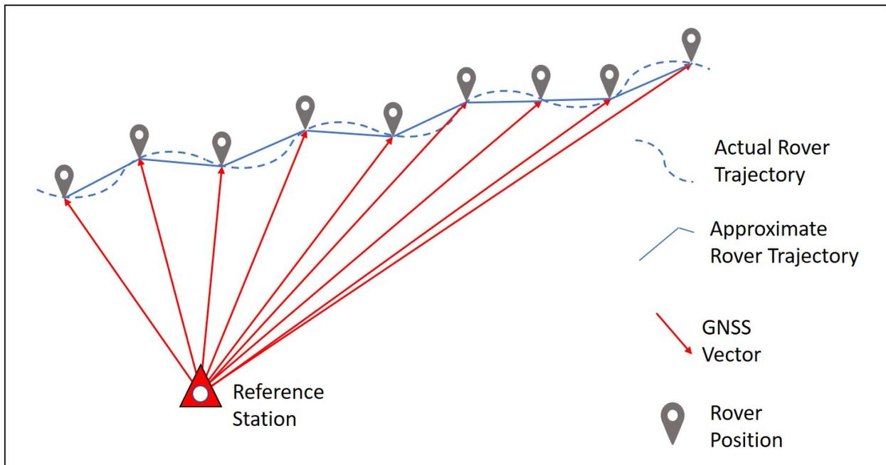
Figure 7: Actual and Approximate Rover Trajectory
