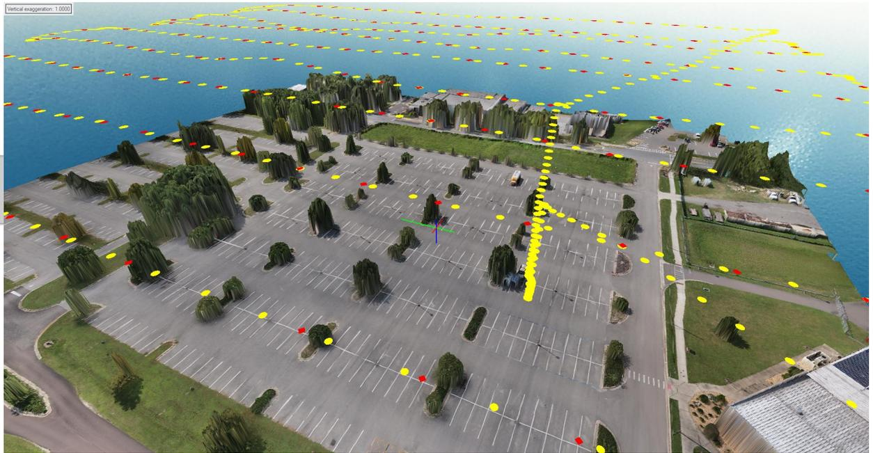
Figure 16: 3D visualization of trajectory points (yellow and interpolated camera exposure positions (red)).
