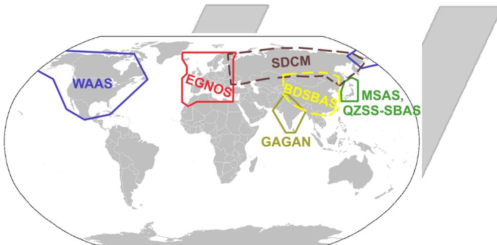
Figure 5: SBAS coverage as of 2018. Source: Persimplex - Own Work, CC BY-SA 3.0, <https://commons.wikimedia.org/w/index.php?curid=18957671>
