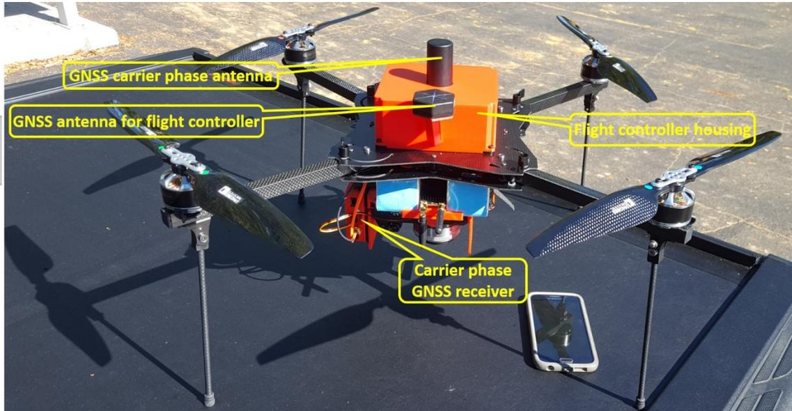
Figure 14: Quad Copter equipped with PPK GNSS for camera exposure event marking.
