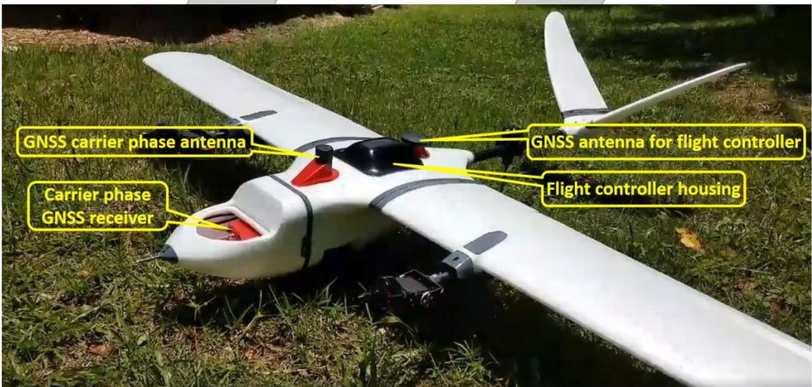
Figure 15: Hybrid VTOL/Fixed Wing platform equipped with PPK GNSS for camera exposure event marking.
