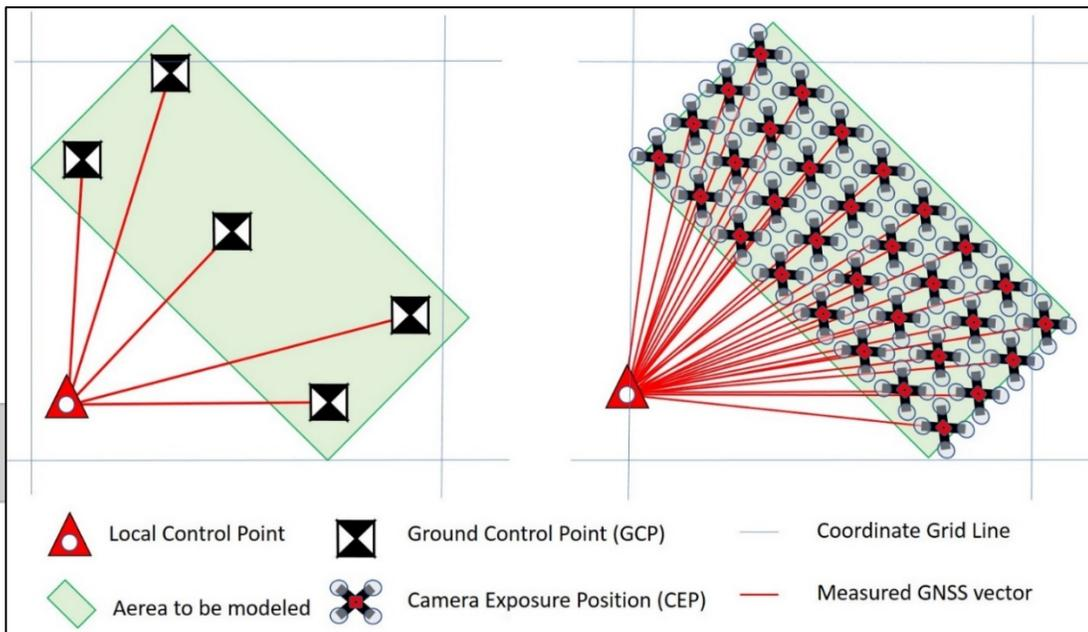
Figure 2: Using a local control point and GNSS measurements to survey ground control points (GCPs) or camera exposure positions (CEPs) for a structure from motion (SfM) mapping project.
