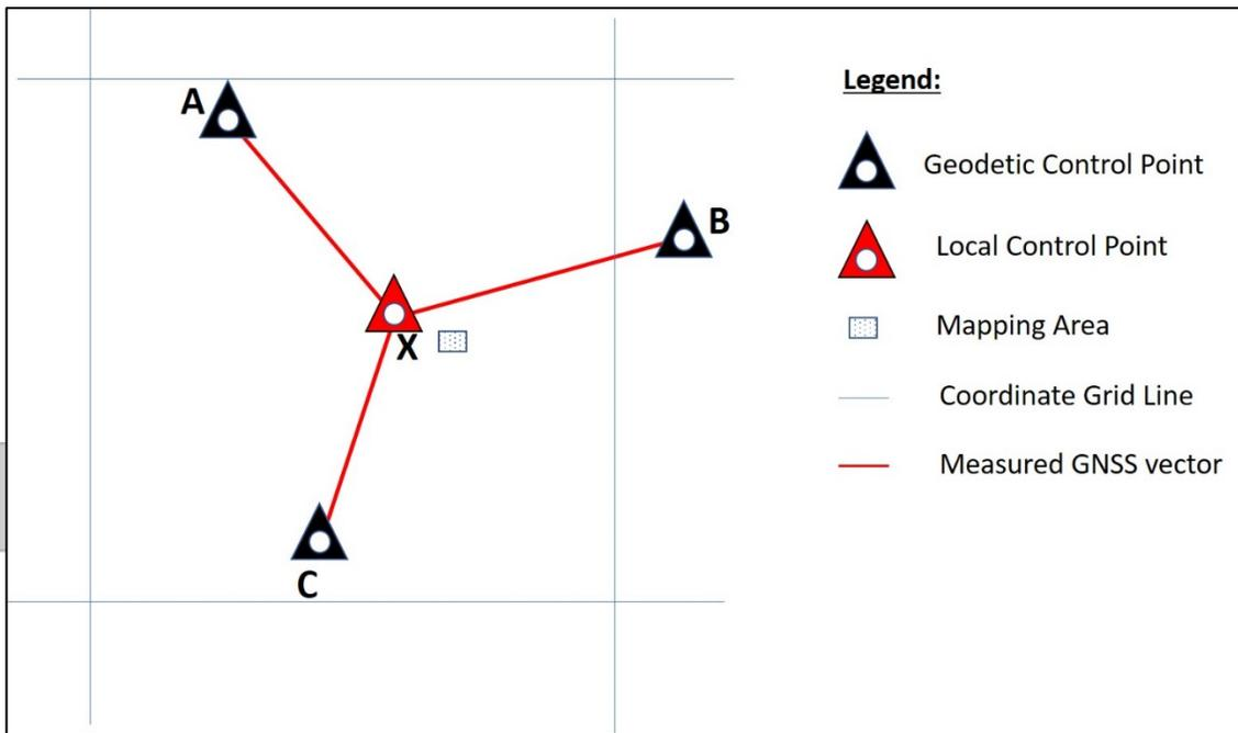
Figure 1: Using a passive geodetic network and GNSS measurements to survey a local control point for a UAV mapping project.
