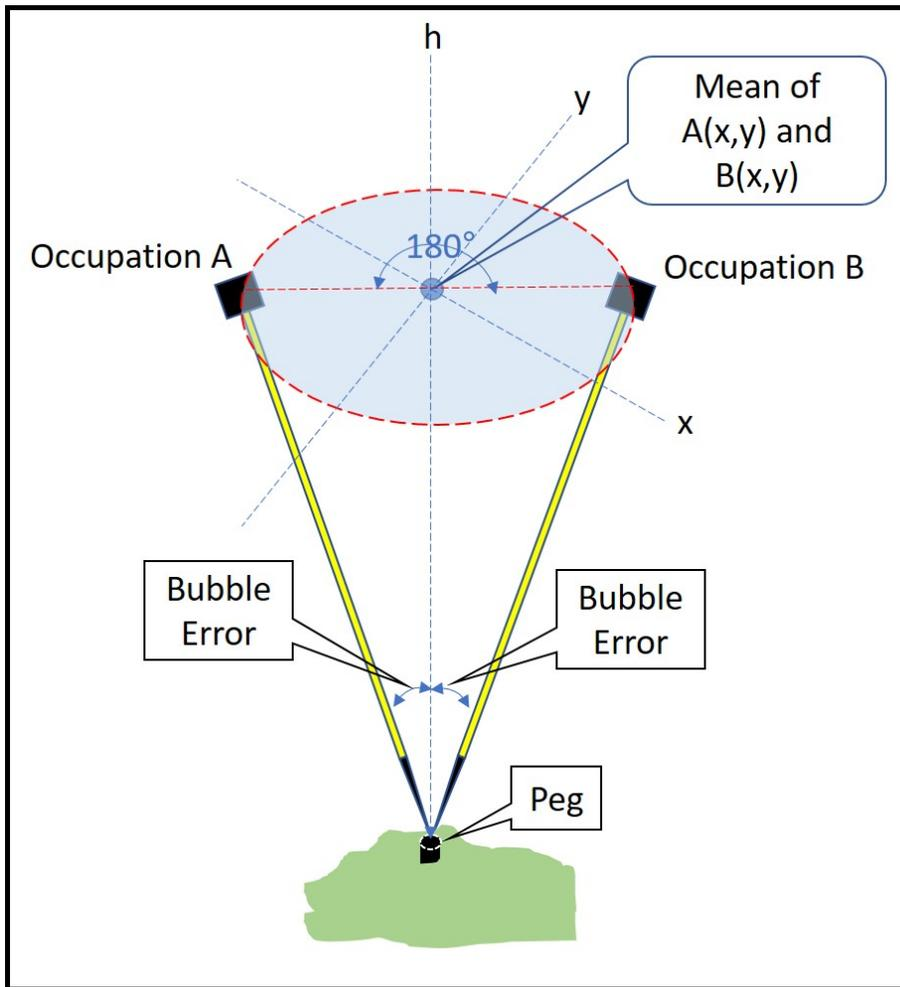
Figure 13: The 180 ° double occupation to eliminate rod bubble error.
