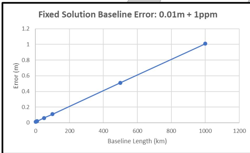
Figure 11: The error of a fixed solution baseline depends mostly on the length of the baseline.
