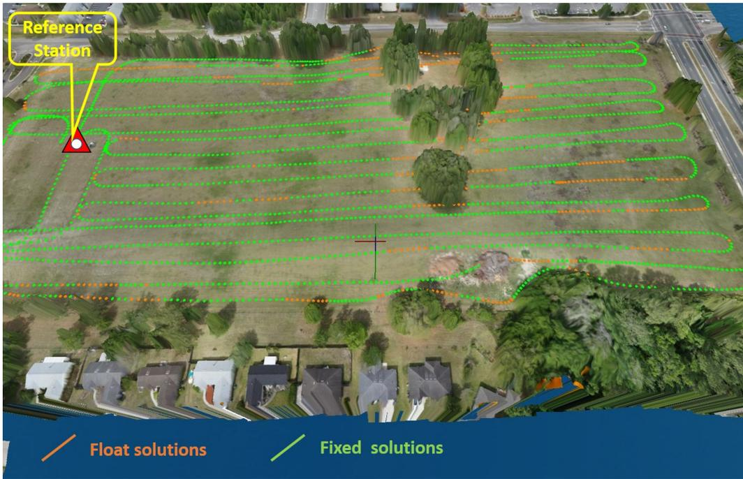
Figure 22: Dual frequency PPK forward **and** backward GPS results (as in RTK) at rover speed of approximately 4m/s. (Approximate field dimensions are 200m x 400 m)
