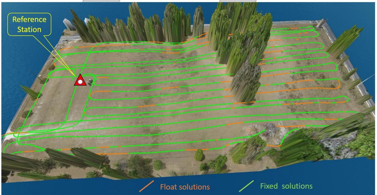
Figure 20: Dual frequency PPK GPS results at rover speed of approximately 4m/s. (Approximate field dimensions are 200m x 400 m)
