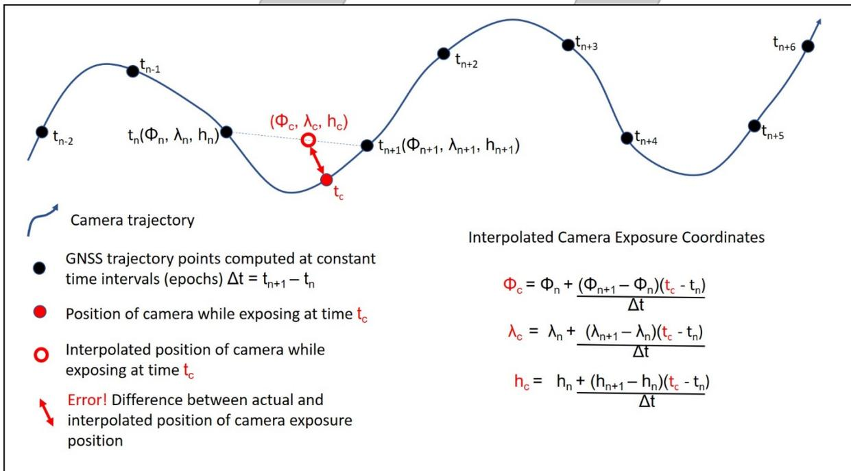
Figure 9: Linear interpolation of camera exposure events.
