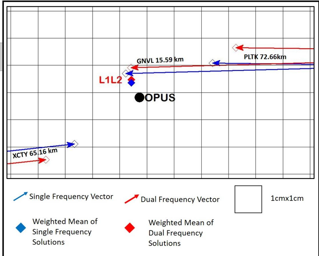
Figure 17: Example of the distribution of single frequency and dual frequency baseline solutions.
