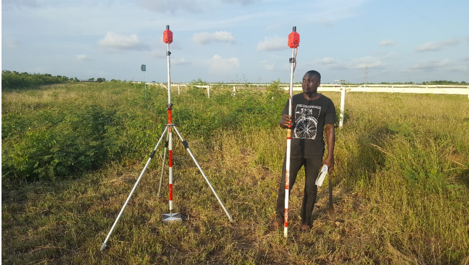
Figure 4: A pair of pole mounted V-Map Systems being employed in a post-processed kinematic survey.
